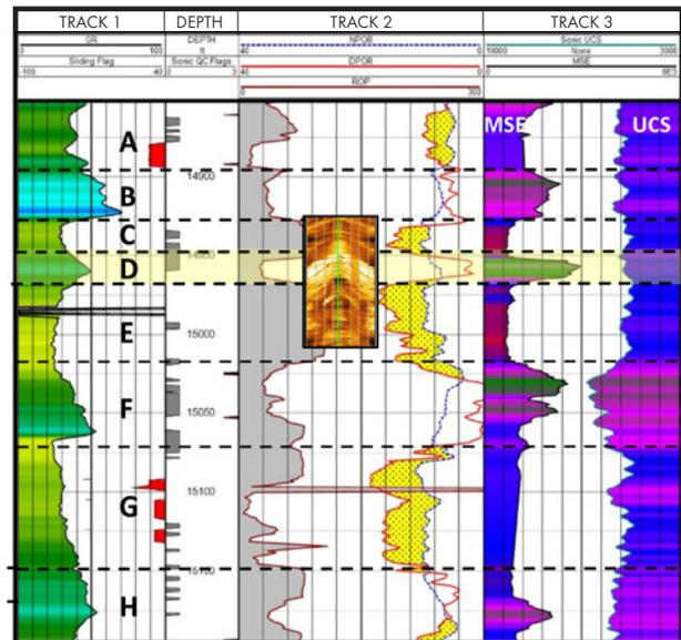
**Interval 4:** In this highly laminated interval, the MSE does an excellent job tracking density log response. In section D, poor sonic quality negatively impacts the UCS result once again.
