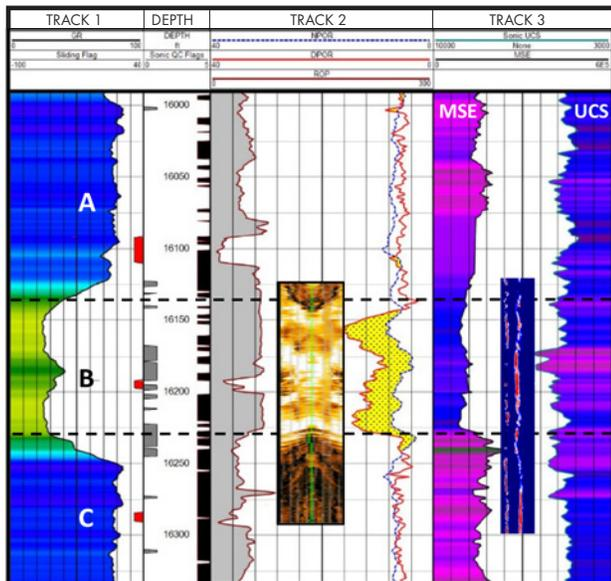
**Interval 3:** The sonic-quality flags shown in the depth track suggest that poor signal-to-noise ratio is preventing UCS from detecting an obvious facies change.
