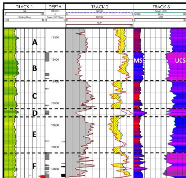
**Interval 2:** Sonic UCS and MSE readings agree with porosity logs. GR is inactive and ineffective in picking up the facies variations.
